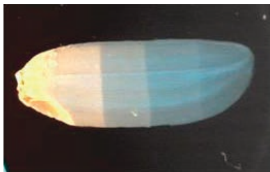
Kernel fissured due to rapid moisture adsorption.
