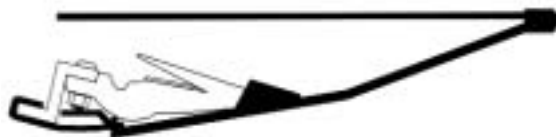
Figure 8-1. Guard extension, usually attached to every other guard, for grain sorghum.
