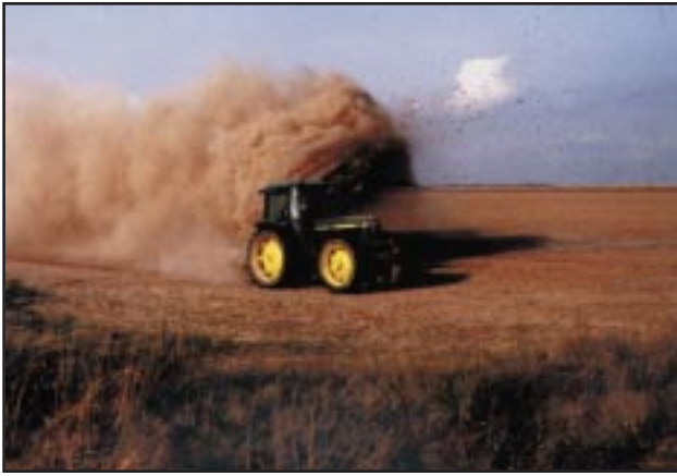
Figure 6.1. A PTO power ditcher is one tool that is used to construct drain furrows for improved surface drainage.
