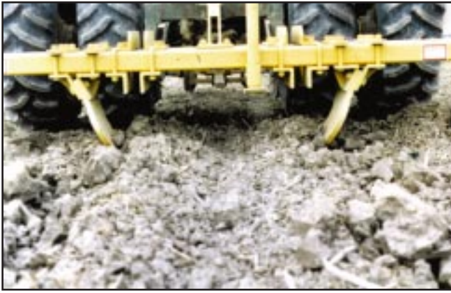
Figure 6.2. Less surface soil disturbance occurs when a high-residue subsoiler is used. This type of subsoiler can be used in no-tillage fields and requires less subsequent tillage in other production systems to adequately prepare the field for seeding.
