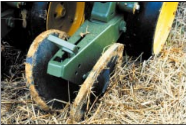
Figure 6.3. Aggressive closing wheels on a planter or soybean drill prevent soil cracking in the furrow before the soybeans sprout.
