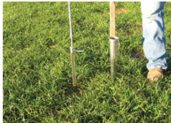
**Figure 10-7. Cone-sampler (left) and core sampler (right) for collection of soil samples.**
