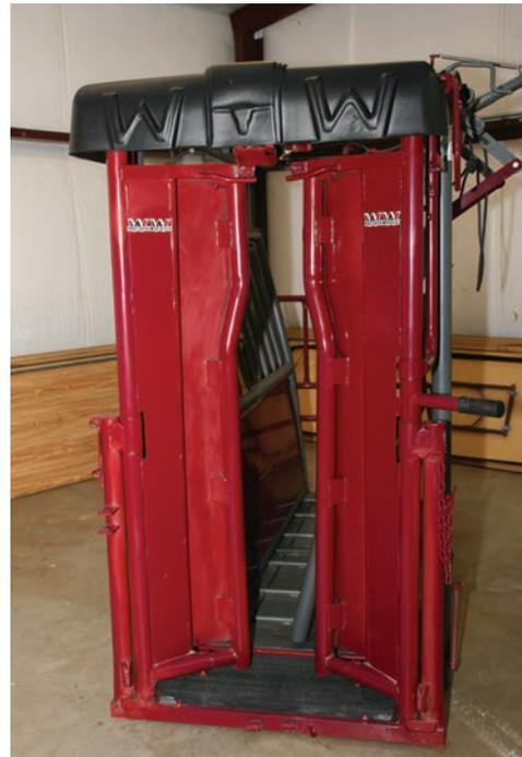
**FIGURE 11-1. All controls are on the front of the chute for one-man operation.**
