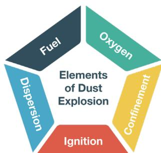
Figure 4. The Essential Elements for Grain Dust Explosion
