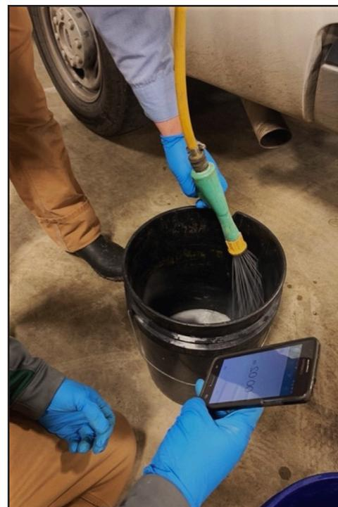
**Figure 1.** Catch test performed using a pre-marked five gallon bucket. Be sure to maintain constant pressure, measure time precisely, and check multiple times to ensure accurate catch test results. Photo credit to Josh Landreth - Ace of Blades, LLC.
