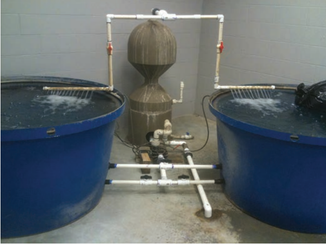
FIGURE 2. An Aquacenter, Inc. two-tank system composed of two 500-gallon polypropylene tanks, a 1/6-hp pump and a bead filter. Note the two parallel pipes between the tanks; on top is the leveling pipe and below is the drain pipe.
