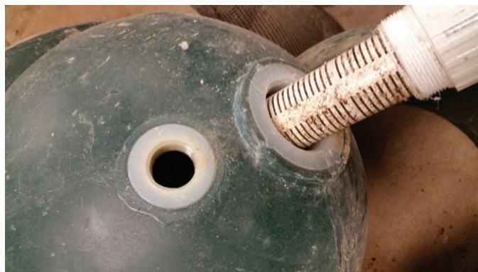
FIGURE 5. Example of the screen in the drain port. A similar screen is used for the water delivery port and the purge port. The open hole is where the 1-inch flexible hose seen in Figure 4 has been detached. There is no screen associated with this hose, and beads will be lost if not used properly.
