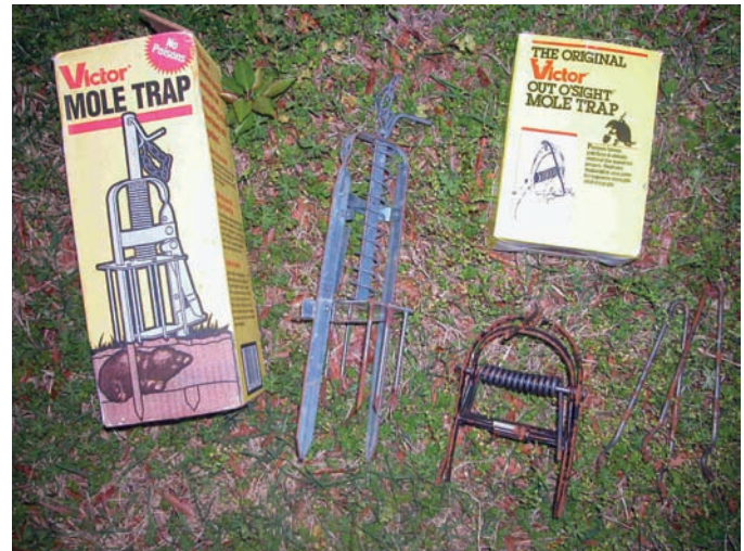
Figure 8. Examples of harpoon- and scissor-style mole traps. Photo by Becky McPeake, University of Arkansas Division of Agriculture.
