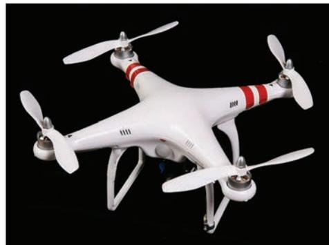
**Example of a small unmanned aircraft system (sUAS).**
