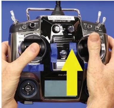
Mode II RC: Pushing pitch/roll stick forward.
