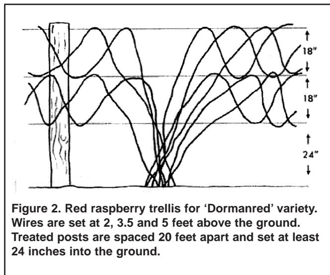
Figure 2. Red raspberry trellis for 'Dormanred' variety. Wires are set at 2, 3.5 and 5 feet above the ground. Treated posts are spaced 20 feet apart and set at least 24 inches into the ground.
