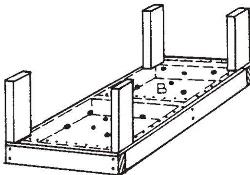
5. Cut four 1-foot lengths from the 16-foot length of 2 x 4 lumber. (Save the remaining 12-foot piece.) Take the two 16- x 42-inch pieces of plywood and place a 1-foot length flat against each short end and flush with the top and side edges. Nail the 2 x 4s in place using 6d nails.
