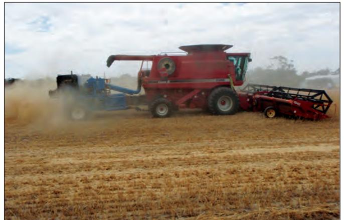
Figure 4. Harrington Seed Destructor used during wheat harvest.
