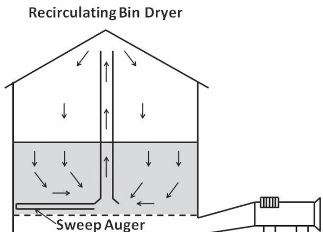
Continuous-flow bin dryers use the same bin setup as the recirculating bins except sweep auger grain is discharged into a cooling bin. High temperature bin drying tends to be more efficient than other high temperature drying processes because the heat is used to dry grain at the drying front which then continues up the grain column to aid in drying before being discharged. (Figure 4)
