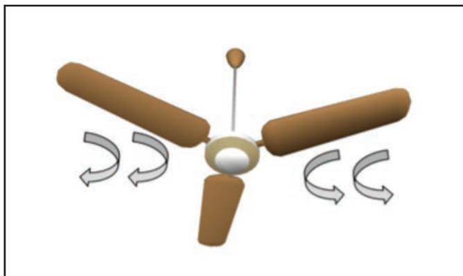
Figure 2. Air movement associated with ceiling fan.
