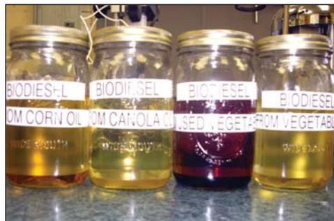
**Figure 1. Biodiesel samples from different plant oils**
