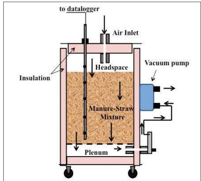
**Figure 3. Biodrying pile preparation.**
