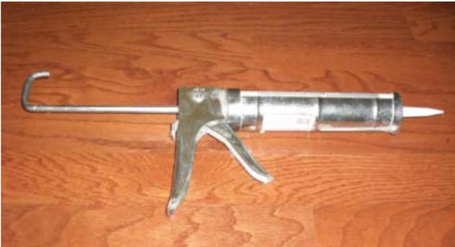
Figure 2. Caulking gun with caulk tube
