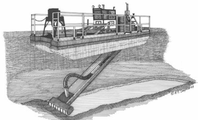
Figure 1. Schematic drawing of a dredge in operation.
