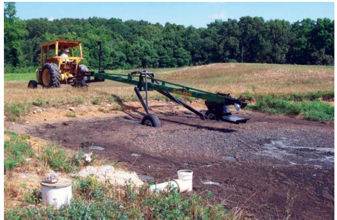
**Figure 3. Trailer-mounted prop agitator with mid-size tractor.**
