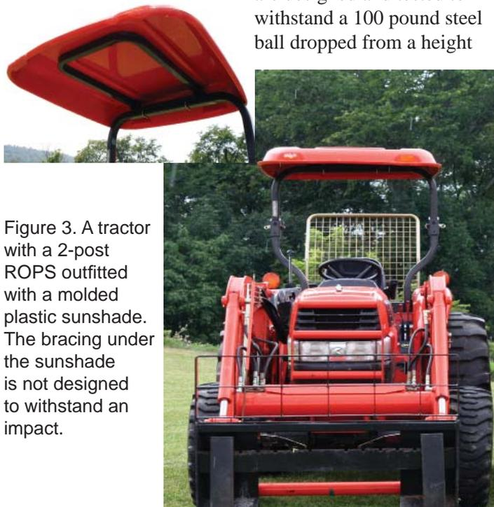
Figure 3. A tractor with a 2-post ROPS outfitted with a molded plastic sunshade. The bracing under the sunshade is not designed to withstand an impact.
