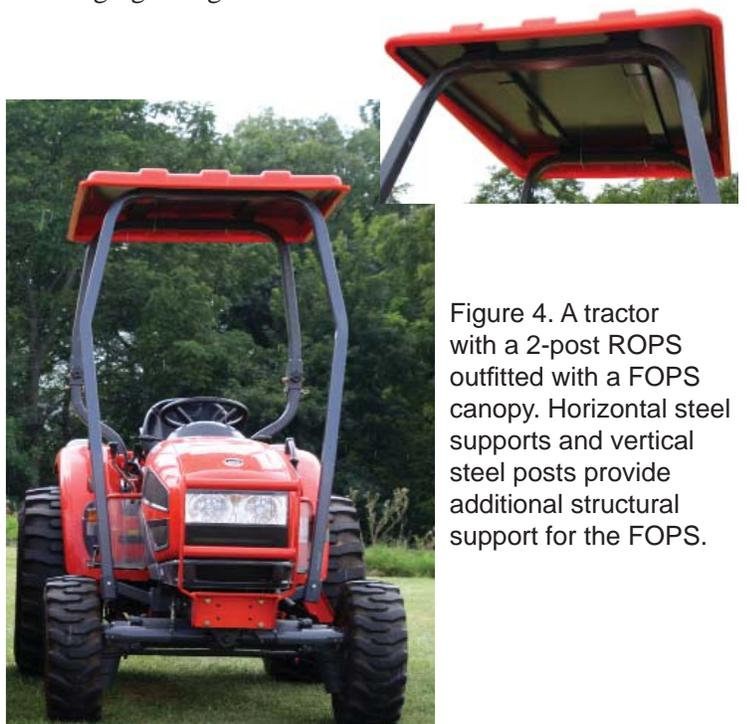
Figure 4. A tractor with a 2-post ROPS outfitted with a FOPS canopy. Horizontal steel supports and vertical steel posts provide additional structural support for the FOPS.
