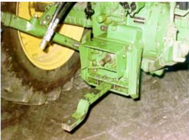
Figure 2. A master shield covering the tractor PTO stub.
