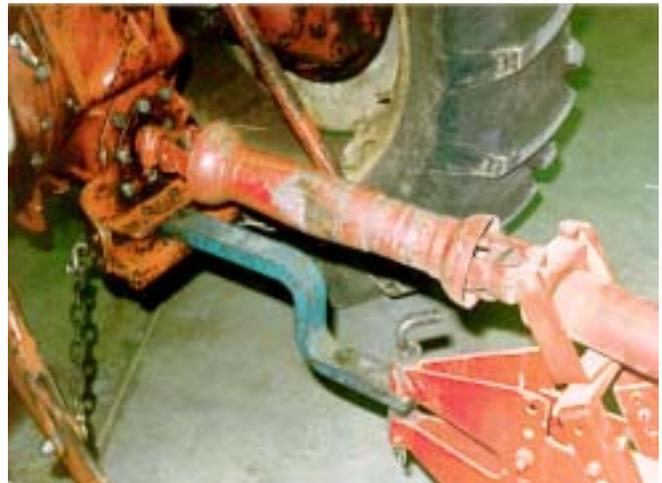
Figure 3. A bent shaft guard offers no protection from a spinning PTO shaft. Also notice the missing master shield and the inadequate guarding of the universal joint near the PTO pedestal. Missing shields and poor maintenance practices often seem to go hand-in-hand.
