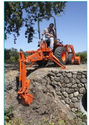
Always operate the backhoe from the backhoe operator's seat.
