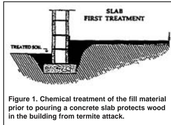
**Figure 1. Chemical treatment of the fill material prior to pouring a concrete slab protects wood in the building from termite attack.**
