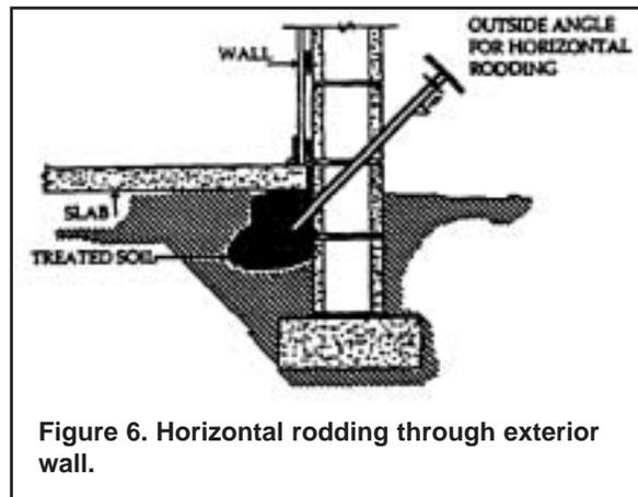
Figure 6. Horizontal rodding through exterior wall.
