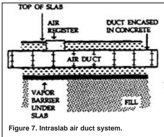
Figure 7. Intraslab air duct system.
