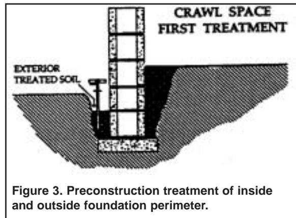
Figure 3. Preconstruction treatment of inside and outside foundation perimeter.
