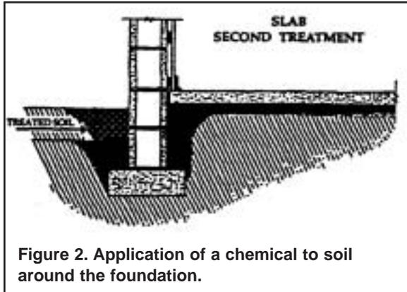
Figure 2. Application of a chemical to soil around the foundation.
