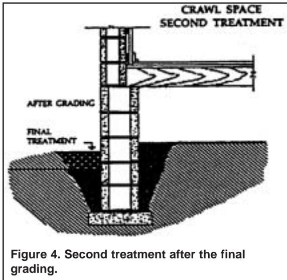
Figure 4. Second treatment after the final grading.
