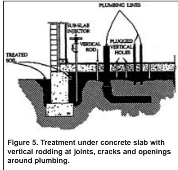
Figure 5. Treatment under concrete slab with vertical rodding at joints, cracks and openings around plumbing.
