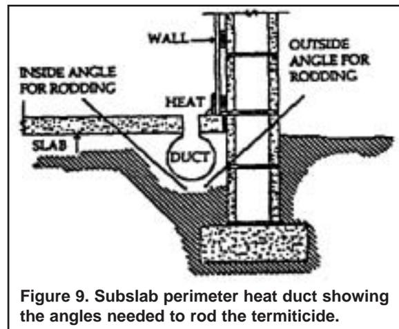
Figure 9. Subslab perimeter heat duct showing the angles needed to rod the termiticide.
