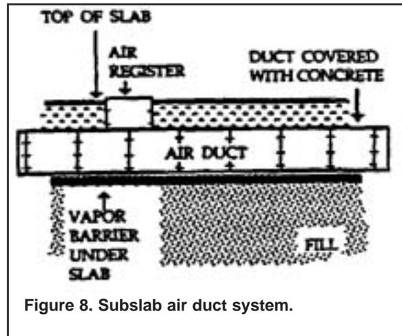
Figure 8. Subslab air duct system.
