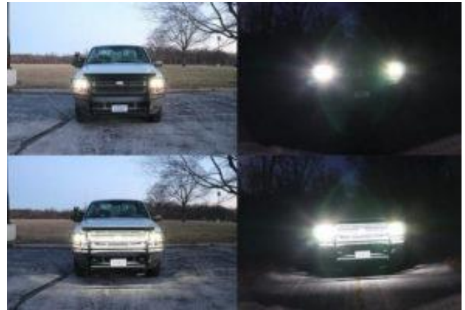
These images from USDA Wildlife Services demonstrate how traditional headlights (top) and the addition of rear-facing LED light bars (bottom) change the vehicle's visibility.
