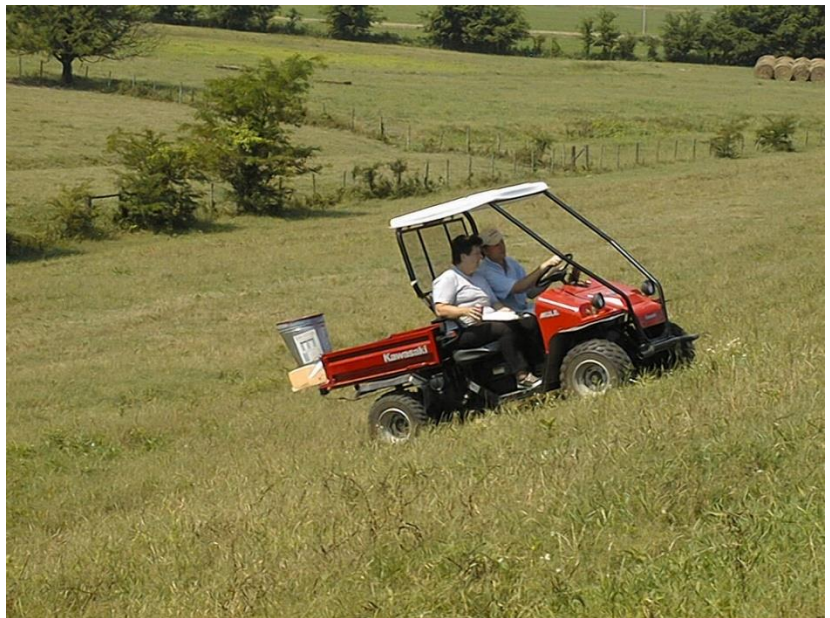
Applying fire ant bait with a Herd seeder attached to an ATV.
