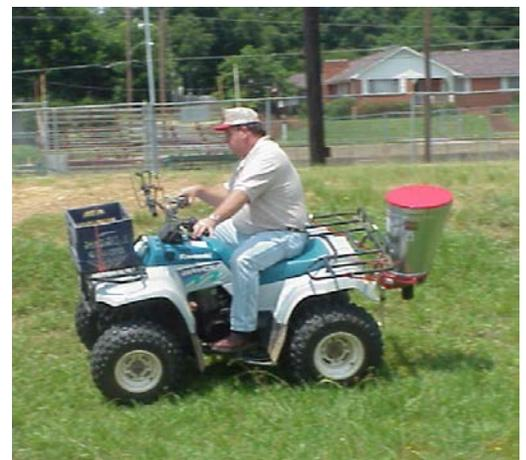
Vehicle Mounted Seeder/Spreader
