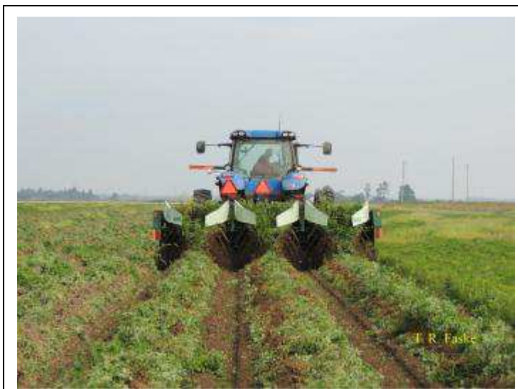
Digging runner peanut with a six-row peanut digger-inverter
