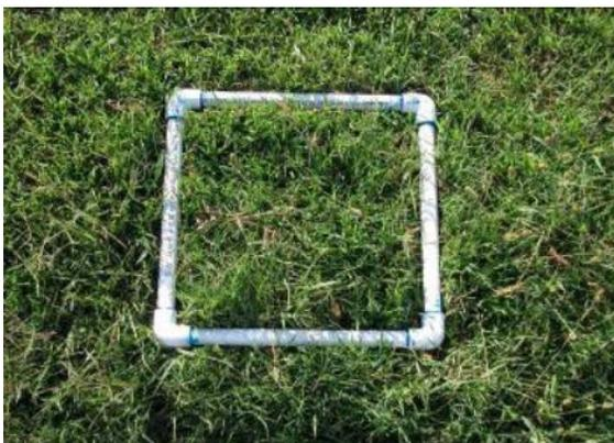
Device used to sample fall armyworm (size: 1 square foot constructed from ½ inch PVC pipe).half-inch PVC pipe).
