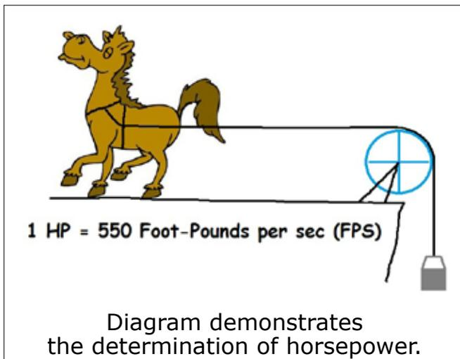
Watt determined that by recording the distance a horse traveled in a specific time while pulling a known weight against gravitational force could measure the power the horse produced. After several observations, Watt concluded a strong horse could provide 550 foot-pounds per second of power.
