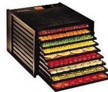
When purchasing, look for double wall construction of metal or high grade plastic with enclosed heating elements. The thermostat should run from 85° to 160° F. and should have a fan or blower. A dial for regulating temperature is good and the unit should have the UL seal of approval.
