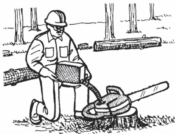
Figure 2. Fueling the Chain Saw.
