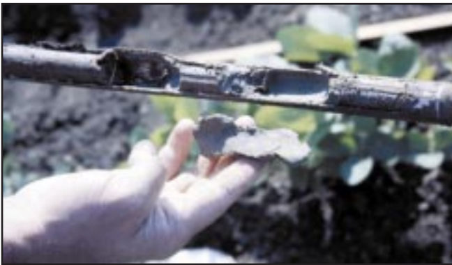
Figure 5.3. A soil sampling tube containing a core of soil to be analyzed.
