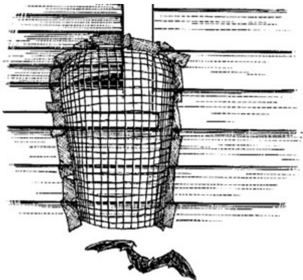
Figure 3. One-way doors allow bats to exit a building but prevent their reentry.
