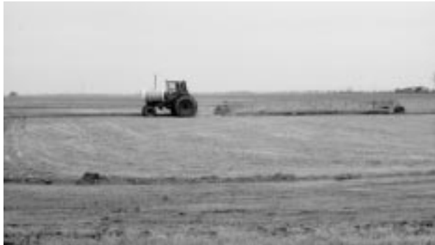
Operation of a land-plane to smooth the field surface and prepare the seedbed.
